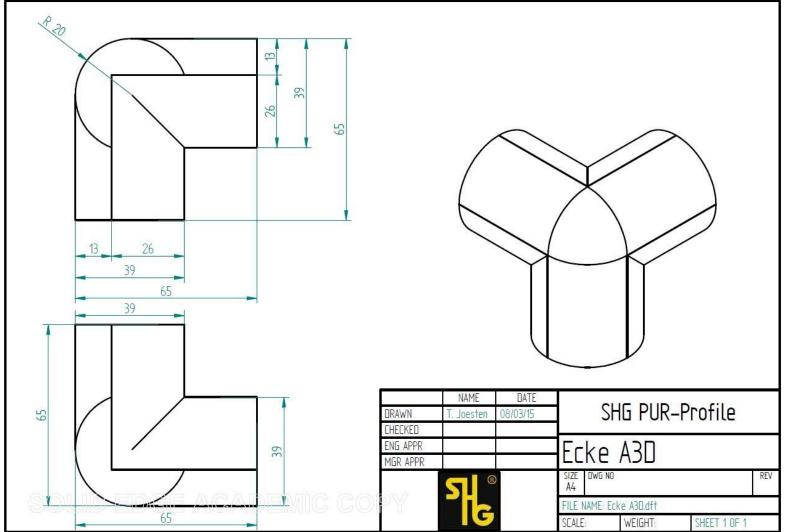
Technical Data Sheet Protective corner, three-dimensional Type A (3D)
